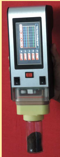
Handheld E-Nose (HEN) with sniffing attachment and sample holder
